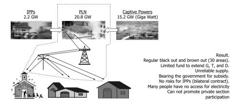
T (Transmission), D (Distribution), G (Generator) IPP = Independent Power Producers, PLN = Electricity State-Owned Company
